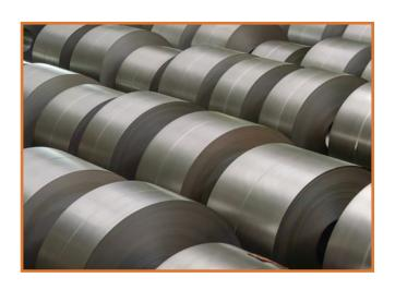
Some of the diverse applications of cold rolled steel include small appliance parts, tool boxes, metal furniture, automobile parts, shelving, lighting, and garages. Cold rolled steels 1008-1010 maintain exceptional versatility for various coatings, good drawability and strength, and all at a cost-effective price.
