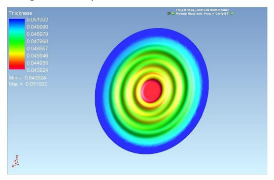
Metal diaphragms are used in a wide array of consumer and industrial applications. Each application has a unique set of parameters that require unique solutions. Hudson has developed the expertise to offer FEA (Finite Element Analysis) with an addition of metal forming software that allows us to create a virtual application environment to test the performance of the diaphragm relative to requirements and predict any metal forming issues due to feature geometry.
