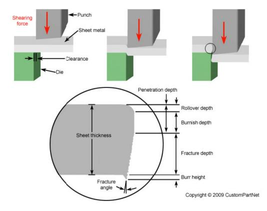
Stamping creates an edge burr. The height, type, and direction of burr are controlled by design, tooling and the equipment used to stamp the diaphragm. The type of material also has a role in edge burr condition. Hudson generally controls burr height to 30% of the actual material thickness. An example would be for .002" thick material, the edge burr would be held to .0006" in height.
