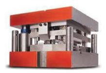
For parts that are <.0015" thick or very high production volume, we consider a high precision metal to metal tool as the best choice. Metal to metal tooling offers the ability for precision alignment to hold exact requirements for burr height, geometry, and very long tool life for working with very thin material and high volume.
