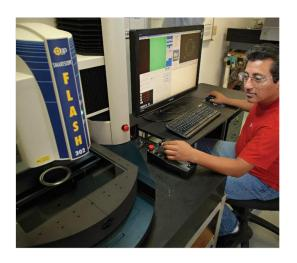
part be laser scanned for dimensions. This usually includes the need for special fixturing and a hold down method that mimics how the part will be restrained in its application in order to measure the part profile.
