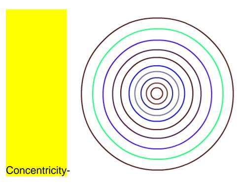
The typical stamped diaphragm has convolutions or concentric rings formed into the part, they control deflection and cycle life. These are controlled by the tooling design and forming method. In order for the diaphragm to perform to design assumptions, the formed rings, inner diameter and outer diameters must run true to one another. We consider normal concentricity to be within .002" for all features on the diaphragm.
