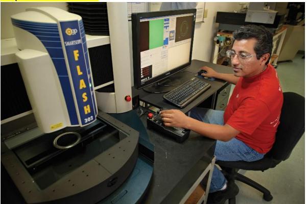
Diaphragms are measured using two main methods; part controlled or die controlled measurements. Because of the delicate nature of most diaphragms, the typical contact method of measuring a feature is not practical due to part alteration from contact pressure. Laser scanning of the part or the actual tooling
